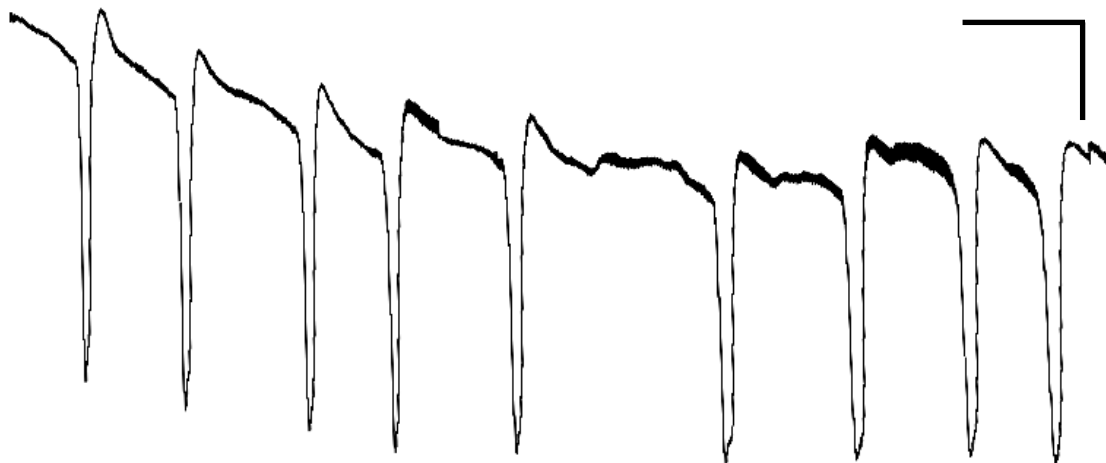
Fig. 3 The tracing showing the DC shift in frontal cortex surface induced by KCl application (Scale bar: 5 min; 10 mV)
