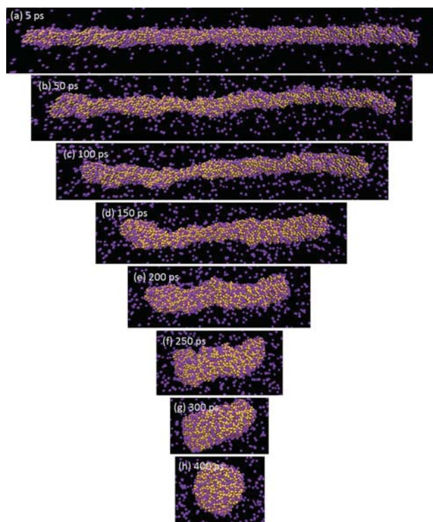
Fig. 7 Coated NW at 1500 K at (a) 5, (b) 50, (c) 100, (d) 150, (e) 200, (f) 250, (g) 300 and (h) 400 ps after initialization. Only the amino groups of AP molecules (violet) are shown for convenience.
