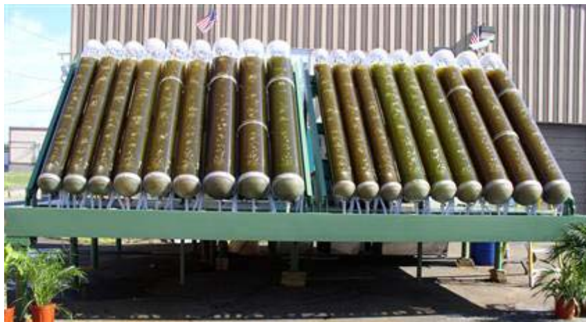
Figure 6 : Algae stored in tubes are busy capturing carbon dioxide in this reactor
