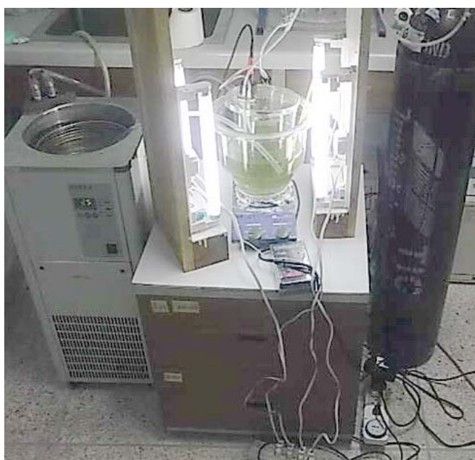
Figure 9. The set apparatus for Botryococcus TRG strain cultivation under batch and semi-continuous regime
