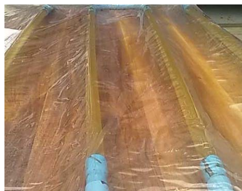
Figure 10. A tubular photobioreactor for Botryococcus TRG strain outdoor cultivation
