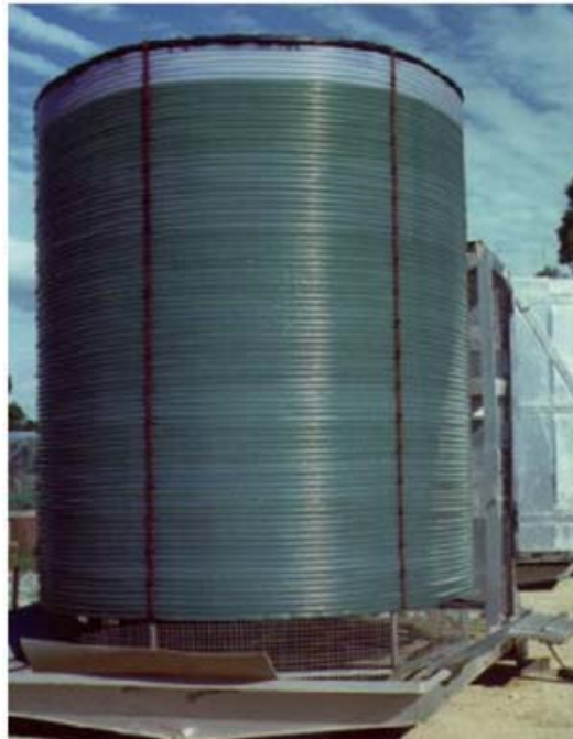
Figure 5 : A 1000 L helical tubular photobioreactor at Murdoch, University, Australia. Source: Chisti (2007)
