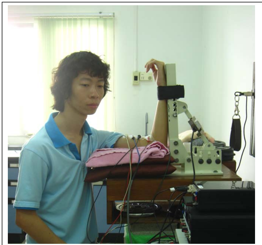
Figure 6 Electrode position to stimulate intramuscular nerve fibres innervating biceps brachii
