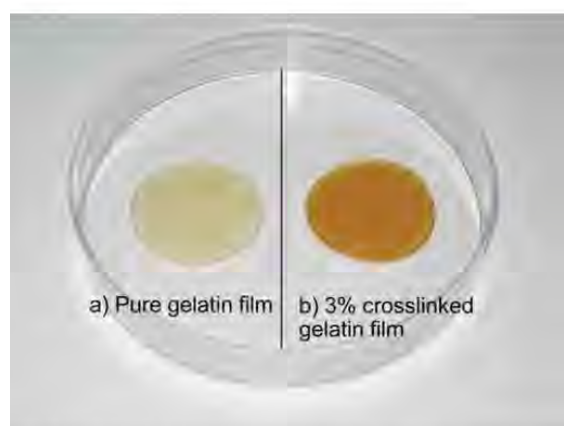
Fig. 2 The image of comparison appearance gelatin films
