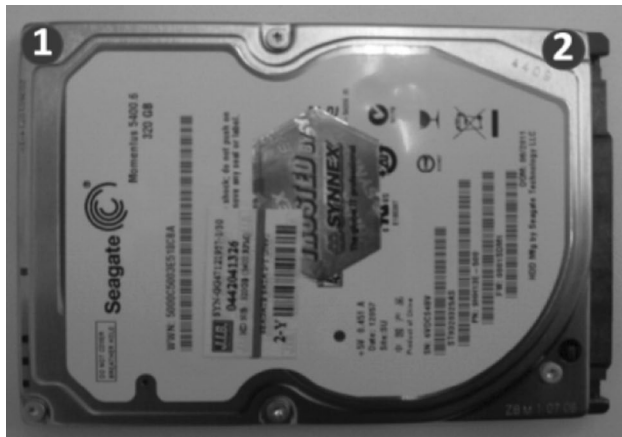
Fig. 1 Vibration measuring positions on HDD case
