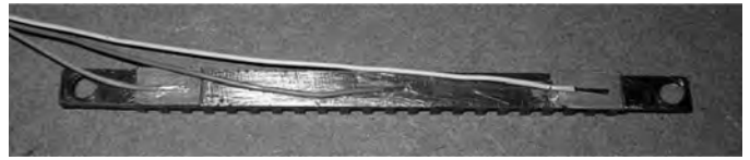
Fig. 7. The linear stator with dual piezoelectric actuators.
