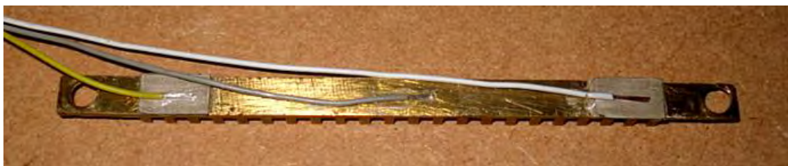
Figure 2.7. The linear stator with dual piezoelectric actuators.
