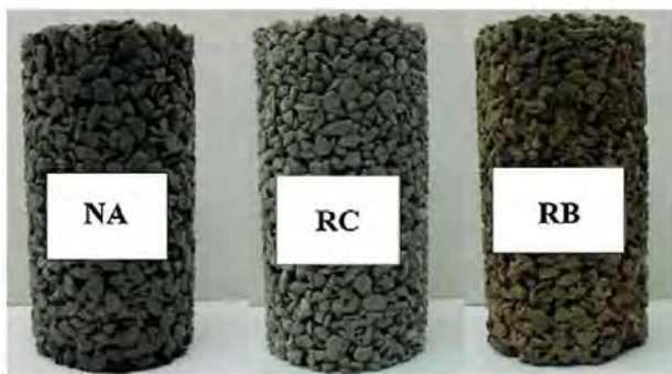
Fig. 2. Specimens of PGC containing NA, RC, and RB after demoulding.
