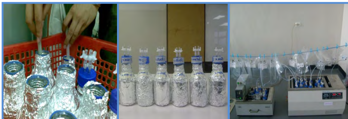
Figure 1. Fermentation process of agro-industrial wastewater for biohydrogen production
