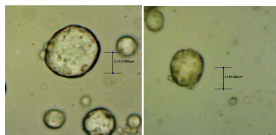
Figure 1. MS-loaded particles in PLA matrix (left) and PBAT matrix (right) using 67.58% HD P(VAc-co-VA) emulsifier
