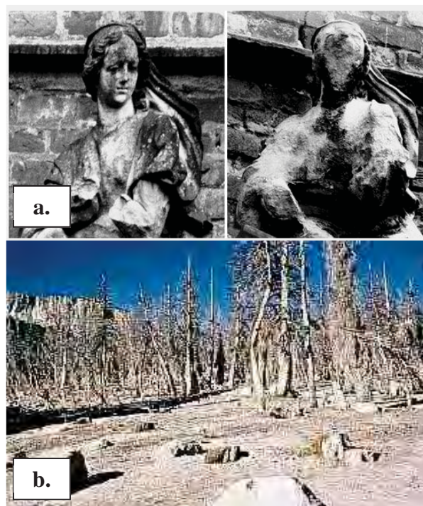
Figure 1 a. Effects of acid rain on stone monument and carvings
