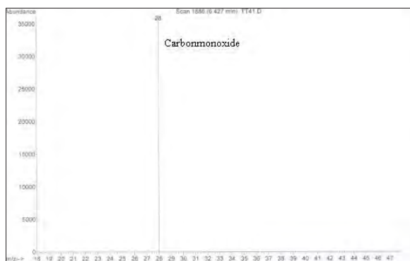
Figure 2. Exemplary EI mass spectrum of CO released from the meat drip of treated tuna sample.
