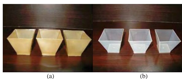
Figure 1. The test samples were prepared by injection molding to a rectangular-shaped tray: (a) pure i-PP and (b) i-PP/MC 20 phr
