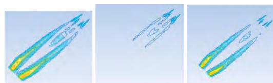
Figure 2. Reaction rate contour of thermal NOx, prompt NOx and N 2 O path (from left to right).
