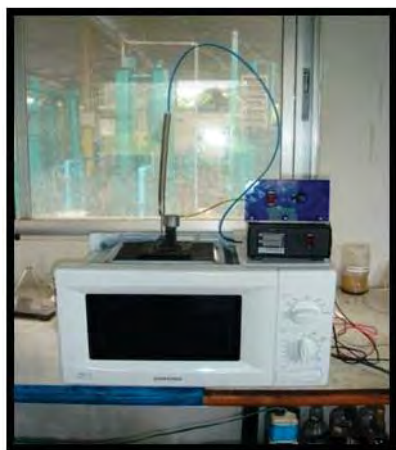
Figure 1. Microwave irradiation-assisted transesterification of tung seed oil.
