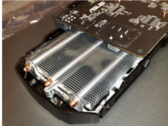
Figure 2.3 Cooling system of an Asus GTX-650 graphics card [20]
