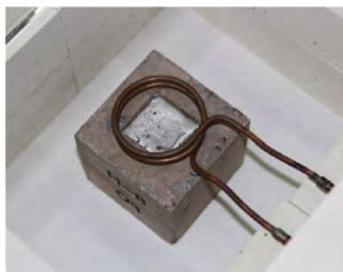
(b) Actual experimental setup (White insulating material on the copper coil was removed for clarity of the heating coil and the LM in the concrete pit)
