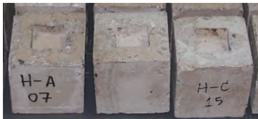
Fig. 7. Examples of fabricated high-density concrete blocks.
