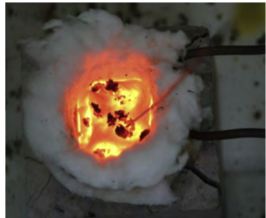
Fig. 8. Red-glowing liquid metal in the concrete block.
