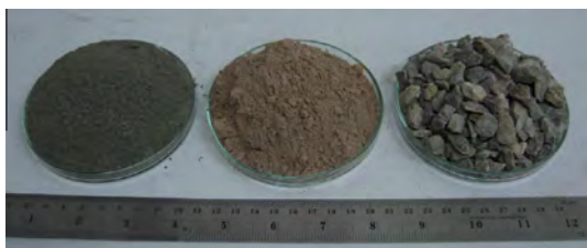
Fig. 2. (From left to right) Examples of cement, fine barite and coarse barite used in this study.
