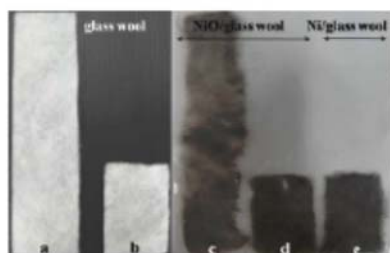
Figure 1. Photograph of glass wool (a,b), NiO/glass wool (c,d) and Ni/glass wool (e) in form of fully and partially packing sheet sizes.
