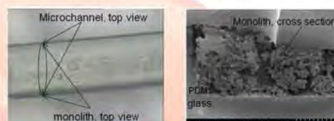
Monolith synthesized in-situ inside microchannel, obtained from microscope (left) and scanning electron microscope (right)
