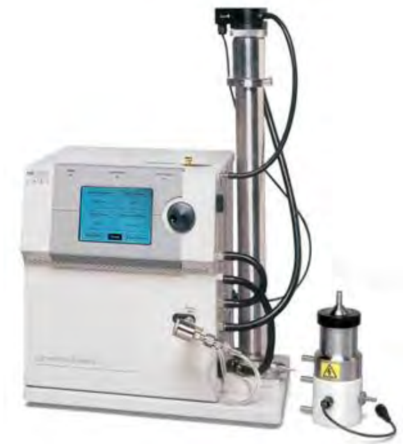
Fig. 2 Particle size distribution measurement device “Series 3080 Electrostatic Classifiers (Courtesy of www.tsi.com )”.
