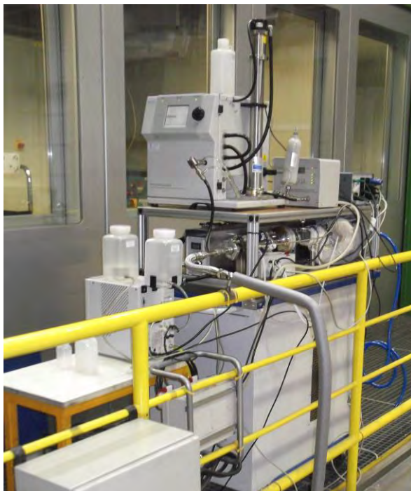
Fig. 3 A Scanning Mobility Particle Sizer (SMPS) for particle size distribution at “Institute for Internal Combustion Engines and Thermodynamics, Graz University of Technology.
