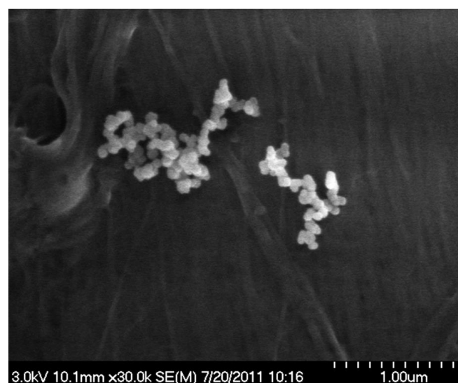
Figure 1. SEM image of fine agglomerated PM emitted from a small diesel engine.
