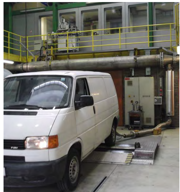
Fig. 1 A diesel van particle emissions test laboratory in “Institute for Internal Combustion Engines and Thermodynamics, Graz University of Technology.
