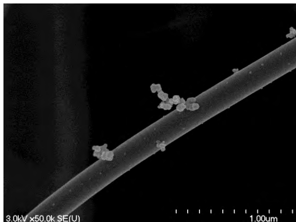
Fig. 6 Scanning Electron Microscope (SEM) images of PMs (Courtesy of Doctoral Thesis, P.Karin Tokyo Institute of Technology).
