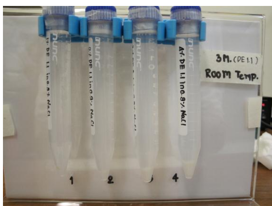
Figure 22 The appearance of tapioca maltodextrin with DE1 solutions on day 1 and 12 th week of storage duration at room temperature and 4 o C.
