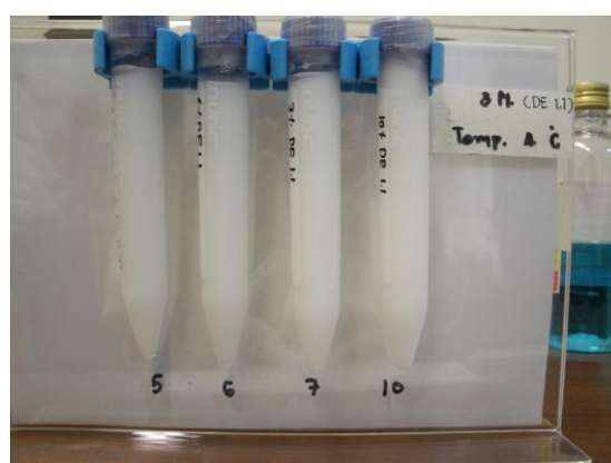
Figure 22 The appearance of tapioca maltodextrin with DE1 solutions on day 1 and 12 th week of storage duration at room temperature and 4 o C.
