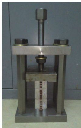
Fig. 3 The loading rig for the applying of sustained loading. Three sensors were pressed in the loading rig at a time.
