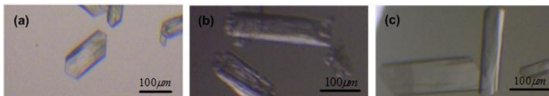
Figure 11. Photomicrographs of seed crystals and product crystals at various times from the growth experiment of form A at 25 °C: seed (a), 30 min (b), 100 min (c).
