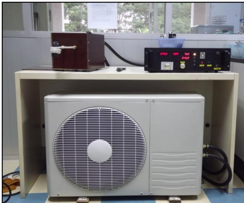
Figure S3 AC EMF generator (AC EMFG) and an induction coil (white coil) to hold vials for induction heating and AC EMF-enhanced dechlorination experiments.
