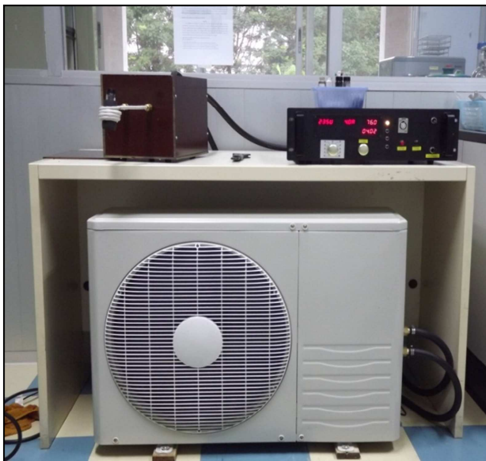
Figure S2 EMF generator (EMFG) and an induction coil (white coil) to hold vials for induction heating and EMF-enhanced dechlorination experiments.
