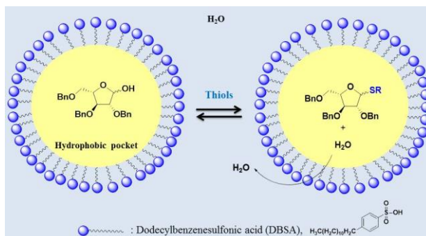
Figure 1. Illustration of dehydrative glycosylation between L-arabinose and thiols in the presence of dodecylbenzenesulfonic acid (DBSA)
