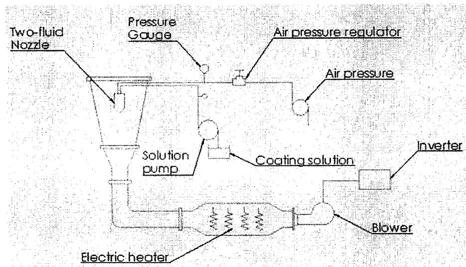
**Figure 1** Schematic diagram of the top-spray fluidized bed coating unit.
