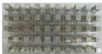
(a) Pure pin-fin heat sink (Model A1)
