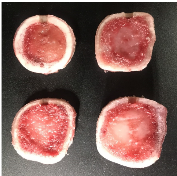
Fig. 13. Cross-sections of drilling holes on four different pieces of femur bones.
