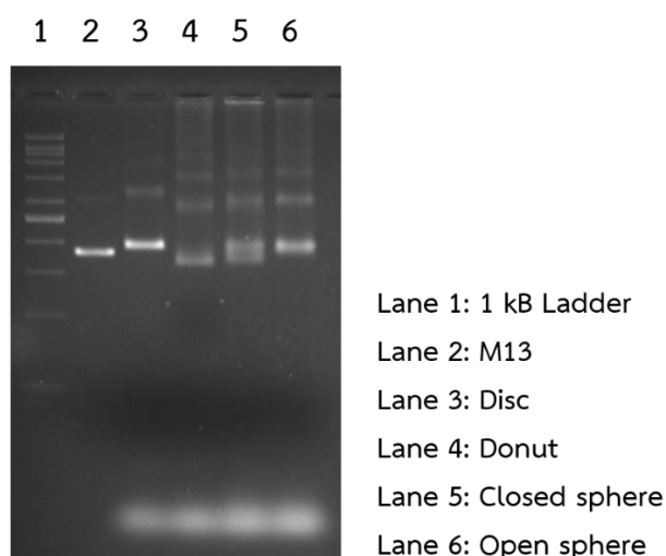
Figure 8 Characterization of DISC, DONUT, and SPHERE shaped DNA origami nanostructures using 1.5% agarose gel. Lane 1 contains 1 Kb DNA ladder, Lane 2 contains M13 scaffold, Lane 3 contains DISC, Lane 4 contains DONUT, Lane 5 contains closed SPHERE, and Lane 6 contains open SPHERE.
