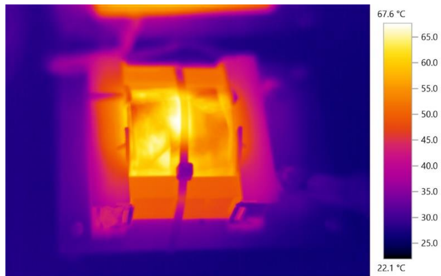
Figure 4-48 Thermal image of the ferrite inductor A after operating at the nominal power 60 minutes.
