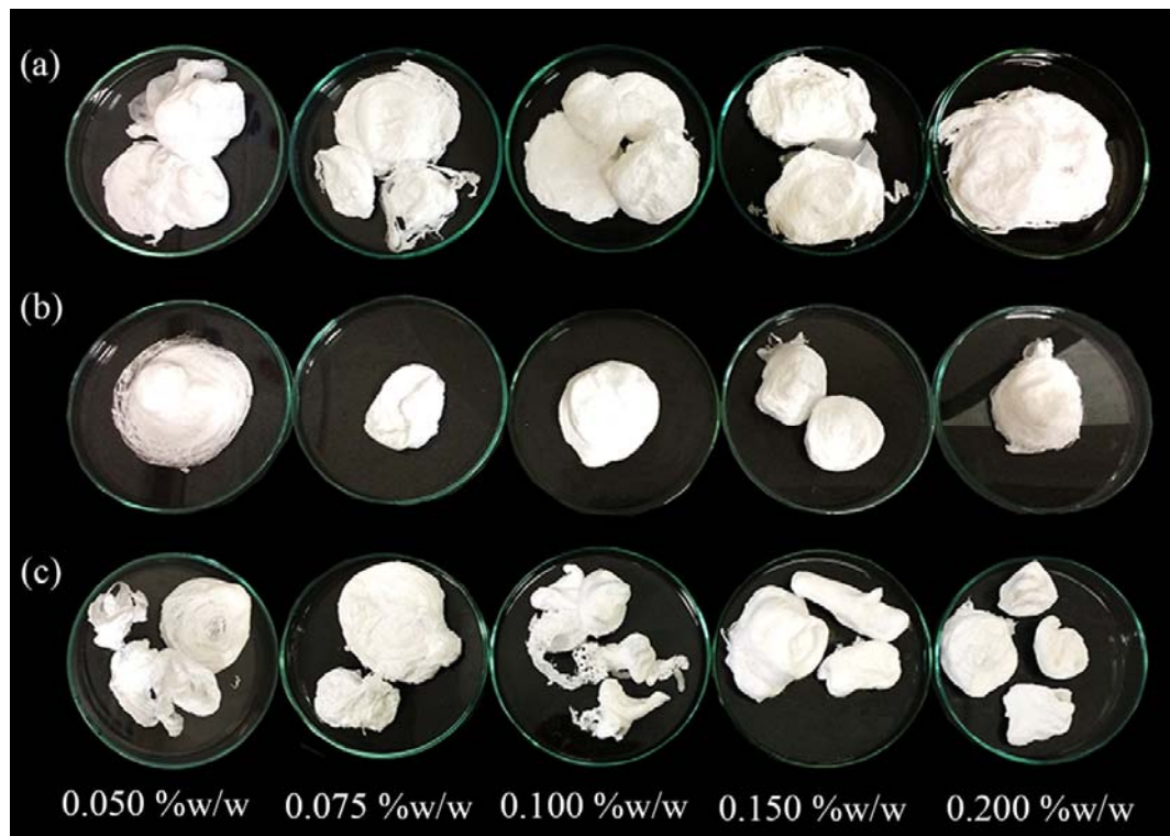
Fig. 14 The physical appearances of purified PCL obtained from the ROP of \epsilon -CL initiated 0.050, 0.075, 0.100, 0.150 and 0.200 %w/w of various initiating systems at 150 °C for 48 h: (a) Sn(Oct) 2 , (b) Sn(Oct) 2 / n BuOH and (c) SnLL4 macroinitiator.
