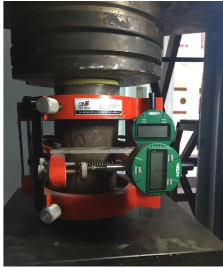
Figure 3.3 Test setup for compressive strength, modulus of elasticity and Poisson's ratio
