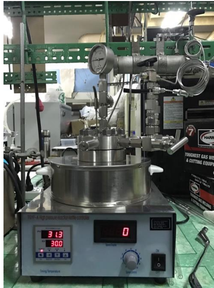
Figure 4. The reaction system for liquid-phase dehydration of ethanol.
