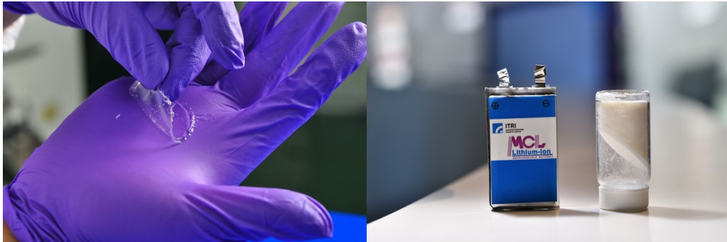
รูปที่ 2-12 Networked Amide Epoxy Polymer Electrolyte for Solid State Lithium-Ion Batteries
