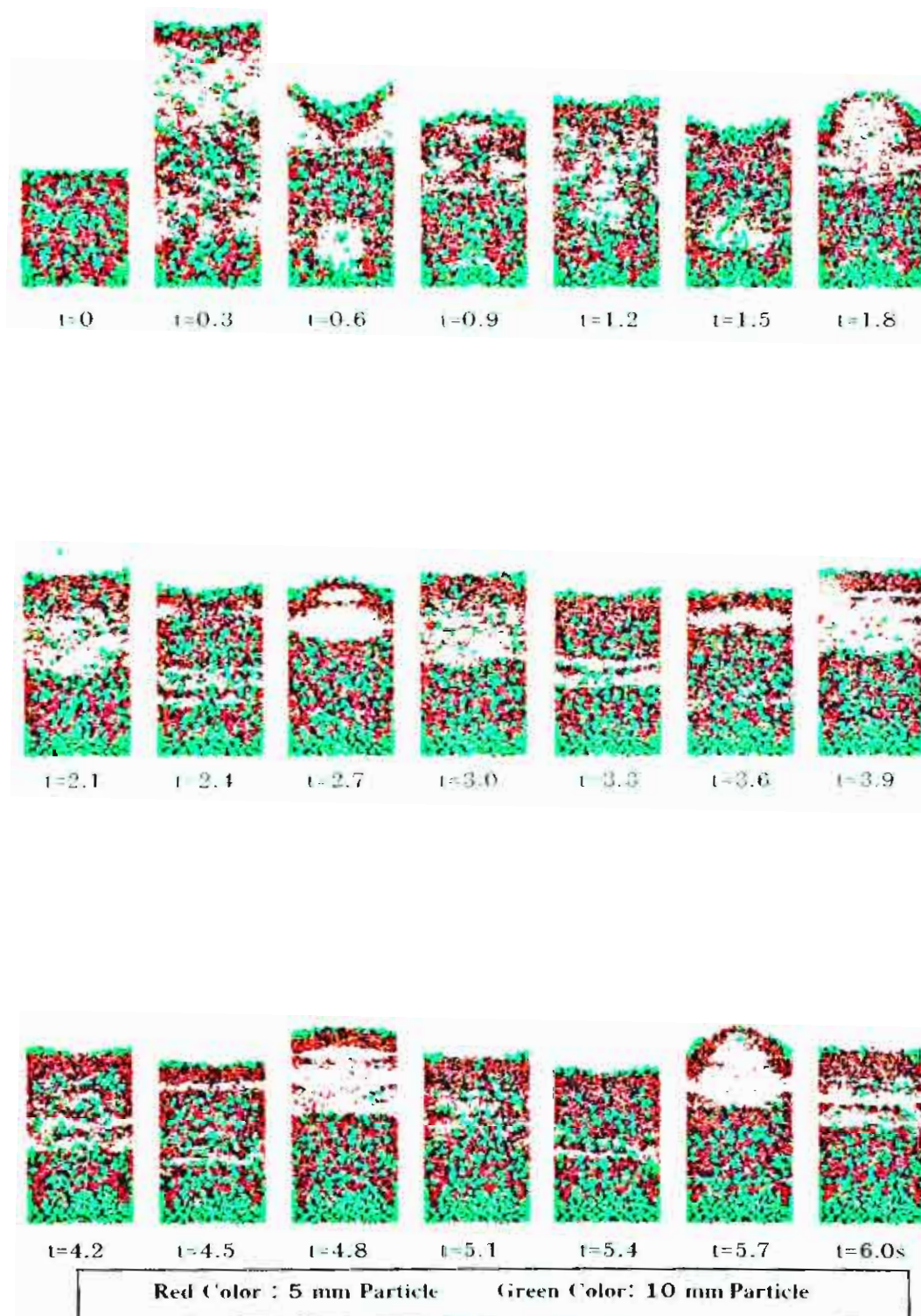
Figure 45. Solids movements at the axially sliced two-dimensional center region, superficial gas velocity = 3.5 m/s, particle size 10mm/5mm ( d_b/d_s = 2.0 )
