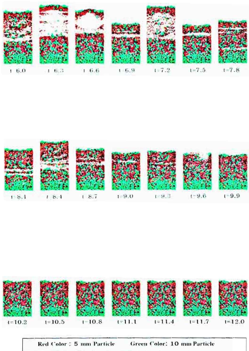
Figure 35. Solids movements at the axially sliced two-dimensional center region, gradually reducing of superficial gas velocity from 3.9 to 2.0 m/s, particle size 10mm/5mm ( d_p/d_s = 2.0 )
