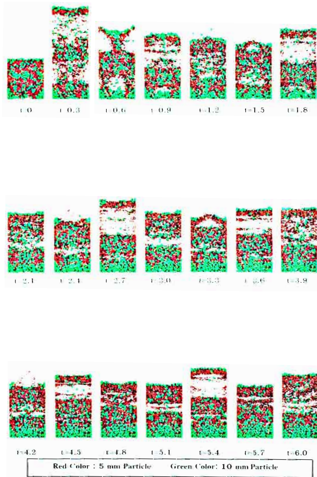
Figure 34. Solids movements at the axially sliced two-dimensional center region, superficial gas velocity = 3.9 m/s, particle size 10mm/5mm ( d_p/d_c = 2.0 )
