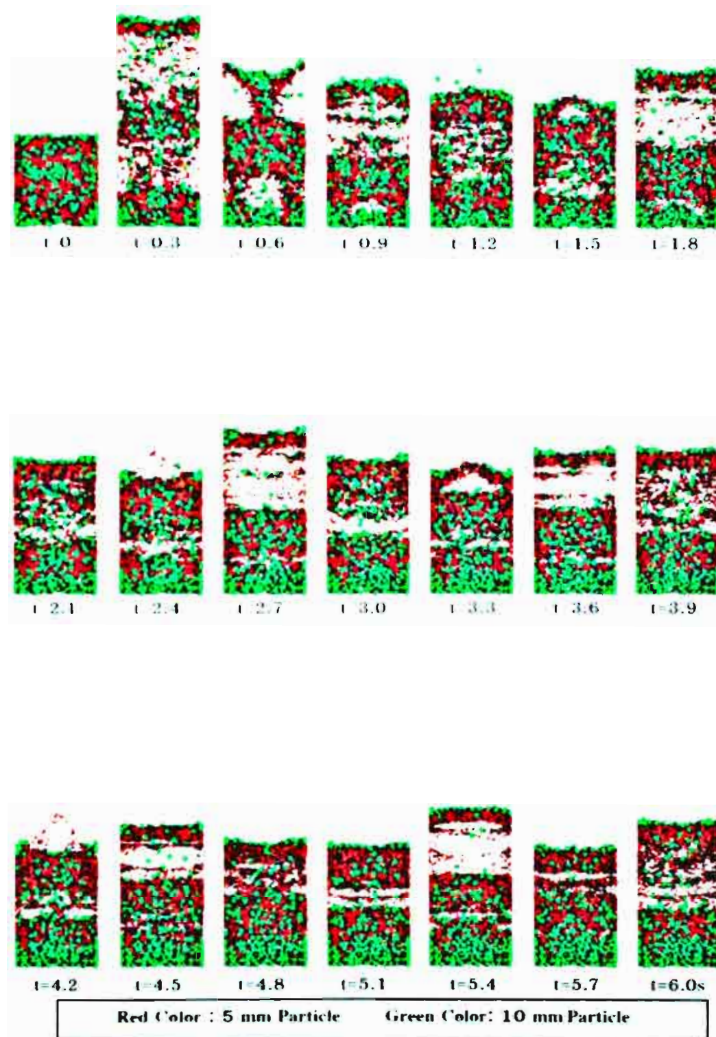
Figure 46. Solids movements at the axially sliced two-dimensional center region, superficial gas velocity = 3.75 m/s, particle size 10mm/5mm ( d_p/d_s = 2.0 )
