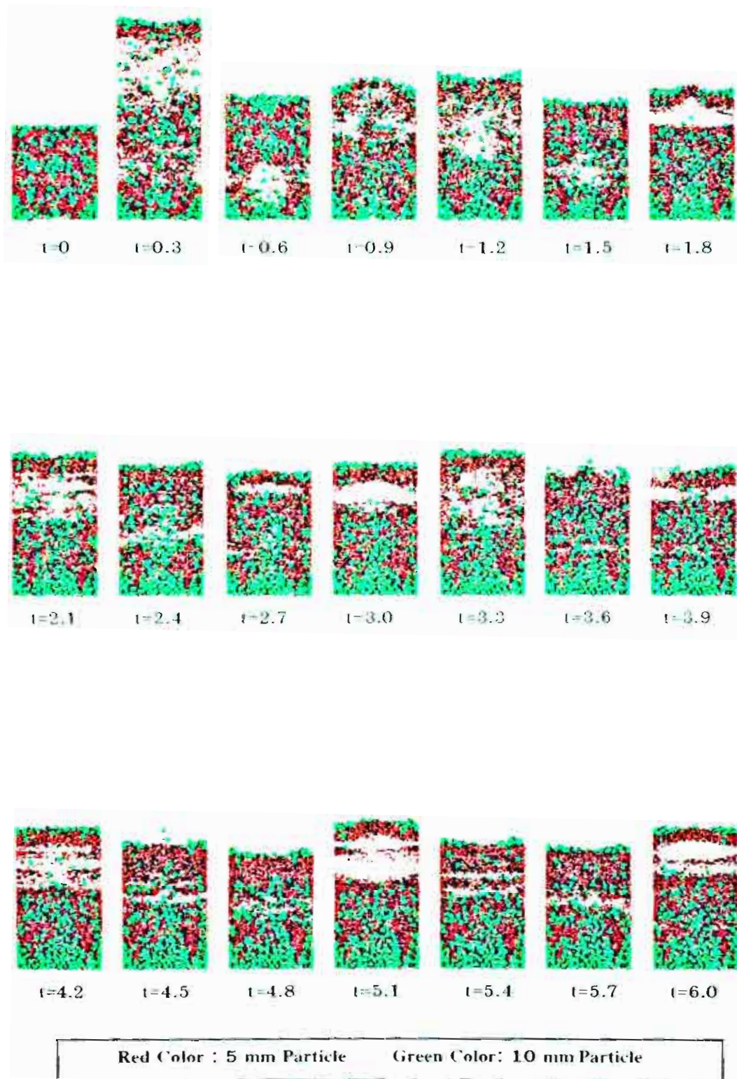
Figure 44. Solids movements at the axially sliced two-dimensional center region, superficial gas velocity = 3.0 m/s, particle size 10mm/5 mm ( d_p/d_c = 2.0 )
