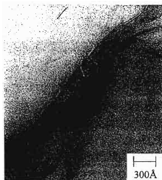
FIG. 5. Transmission electron micrograph of DDA-clay aggregates in a melt-processed sample.
