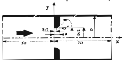
Fig. 1 Geometry of pipe with the orifice.
