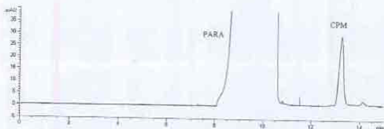
Fig. 3. A representative electropherogram of PARA and CPM in brand A. Other conditions are as Fig. 4.
