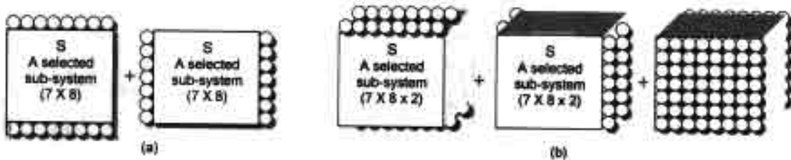
Figure 61: Some examples of a selected sub-system (S) and all of its corresponding CUs at boundary of S: a) all CUs for a 2-D mesh sub-system ( N' = 7 \times 8 ) and b) all CUs for a 3-D mesh sub-system ( N' = 7 \times 8 \times 2 ).
