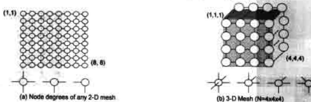
Figure 85: Node degrees: a) at most 4 for the 2-D meshes and b) at most 6 for the 3-D meshes.
