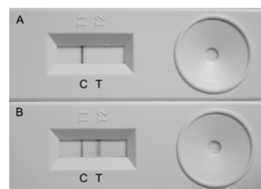
Fig. 1 Detection of NoV in a stool sample by using the IP-Noro kit. The test is negative when only one line appears in the control area (A). The test is positive if two lines appear in the membrane (B).
