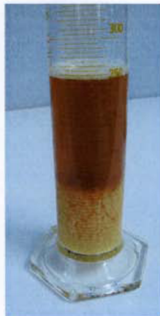
Sedimentation of flocculent
