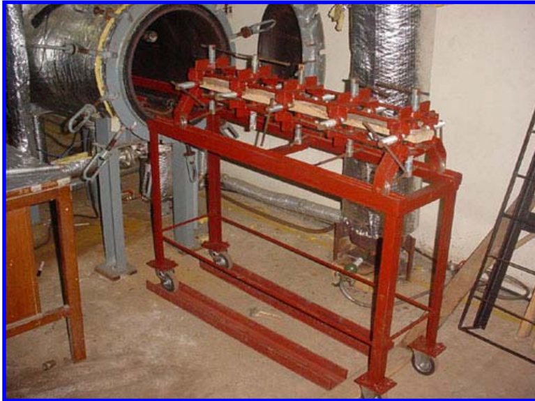
Figure C.4: Roller designed to straighten wood and reduce cracking.
