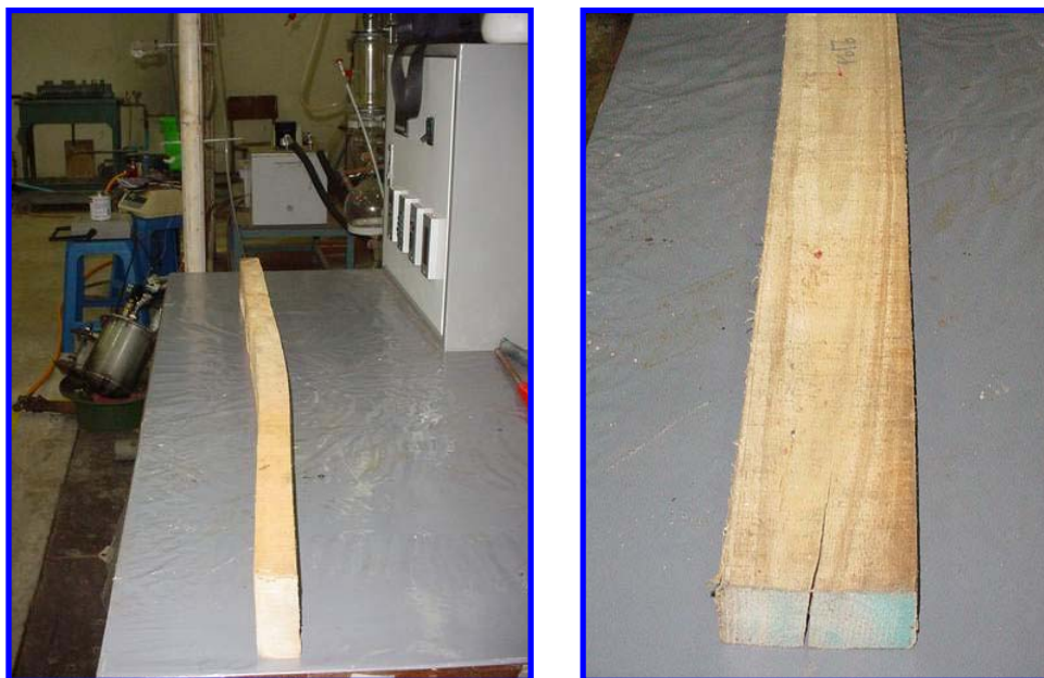
Figure 4.5: Examples of unacceptable pieces of dried wood showing (a) warp and (b) fracture.
