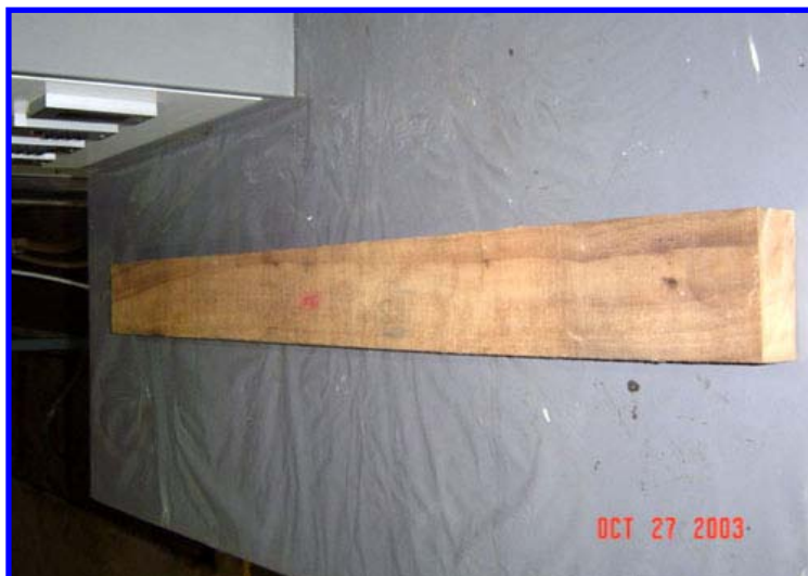
Figure C.8: Top view of board Grade C after drying at optimum condition.
