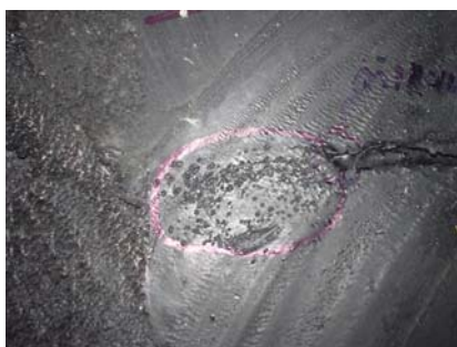
Figure 3 Sample with porosity
