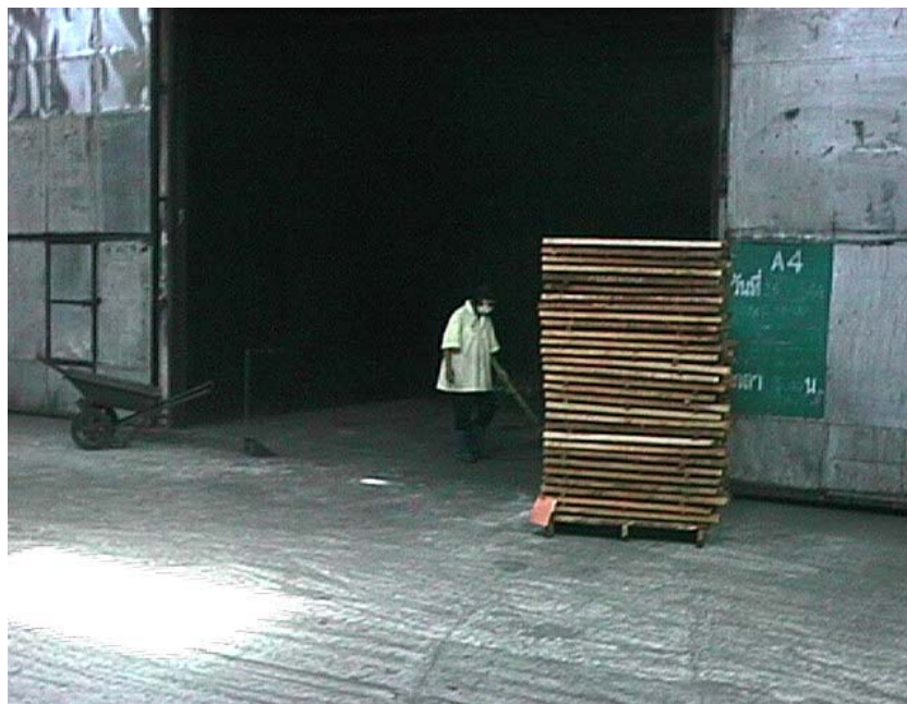
Figure 2.9: Stacks of lumber are placed in the drying kilns and dried at 80-100°C.
