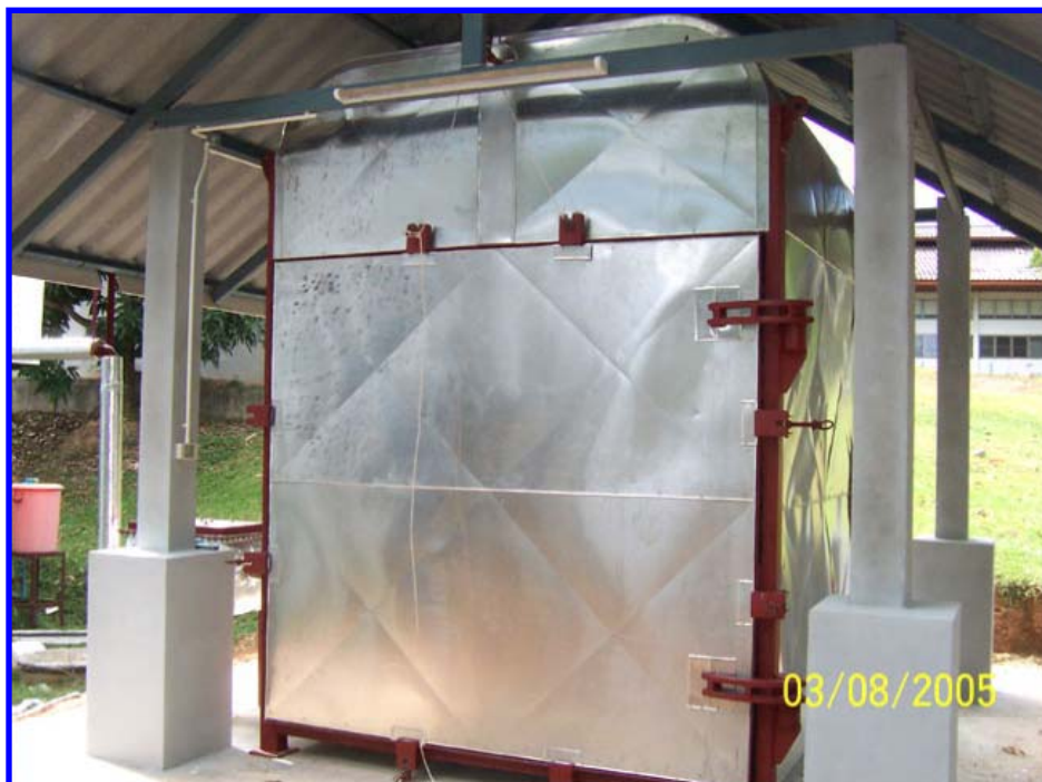
Figure 3.2: The 2.4 m x 2.4 m x 2.4 m drying kiln.
