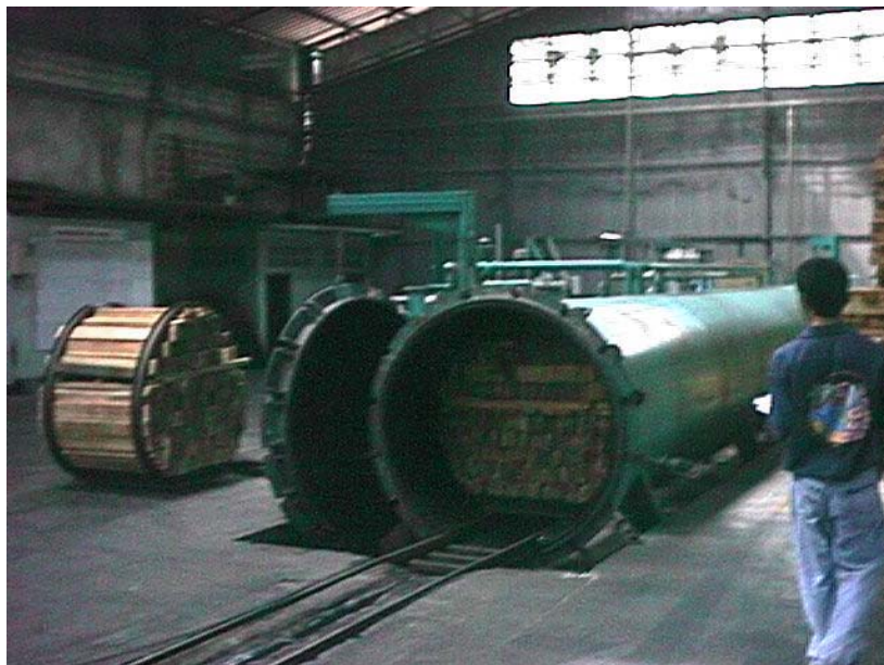
Figure 2.7: Treatment of lumber with boron salt to prevent insect attacks.
