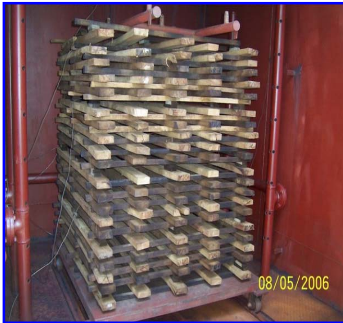
Figure 3.11: Wood is clamped and placed inside the chamber. (This operation was done in the latter stages of the research).
