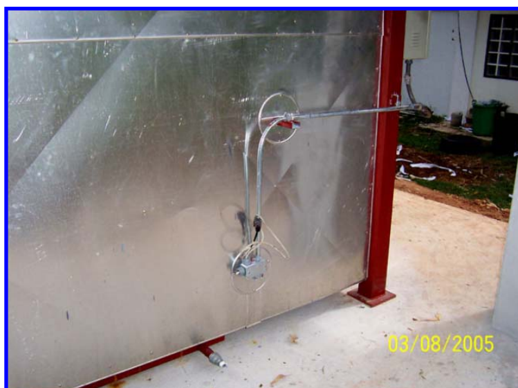
Figure 3.6: A steam trap and a water drain at the bottom of the drying kiln.
