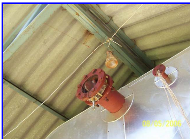
Figure 3.4: A vent located at the top of the drying kiln for removing moisture. To the right is the insertion point for thermocouples.
