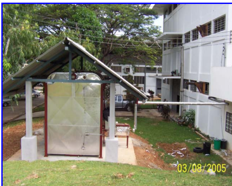
Figure 3.3: The drying kiln located just outside the Department of Chemical Engineering, Faculty of Engineering, Prince of Songkla University. The picture shows a steam pipe running from the boiler inside the building.
