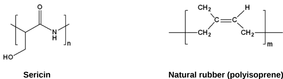
Figure 2 Chemical structures of sericin and natural rubber.
