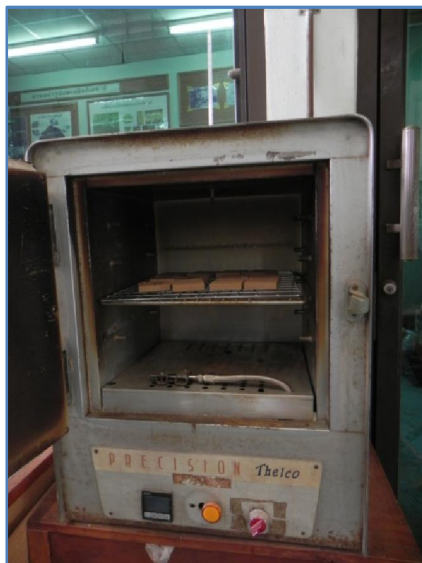
Figure 1-24 and 1-25 Density and moisture content test
