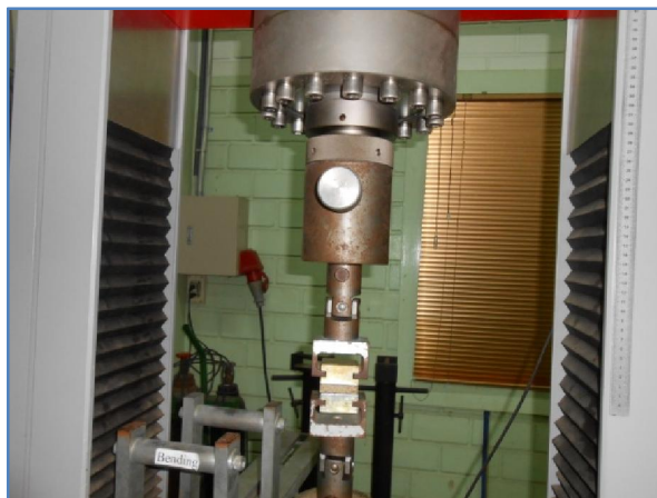
Figure 1-29 Internal bonding test
