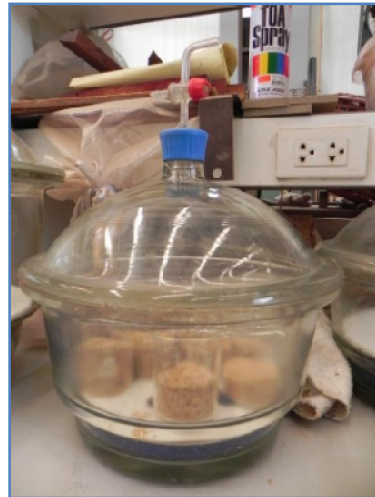
Figure 1-13 and 1-14 Moisture content of rubber wood fiber measuring
