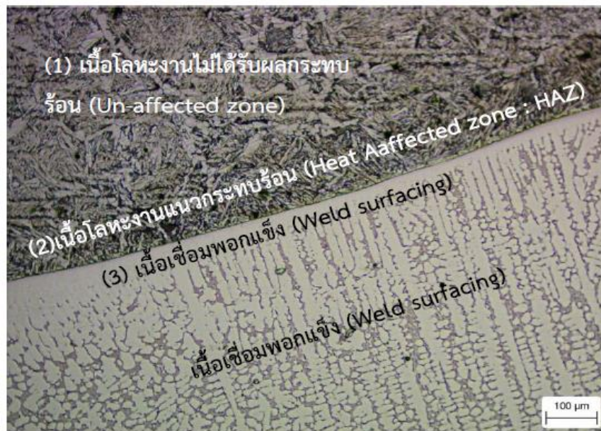
Weld Structure : Magnification 50X
