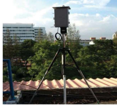
Figure 3. Portable single-frequency base station.
