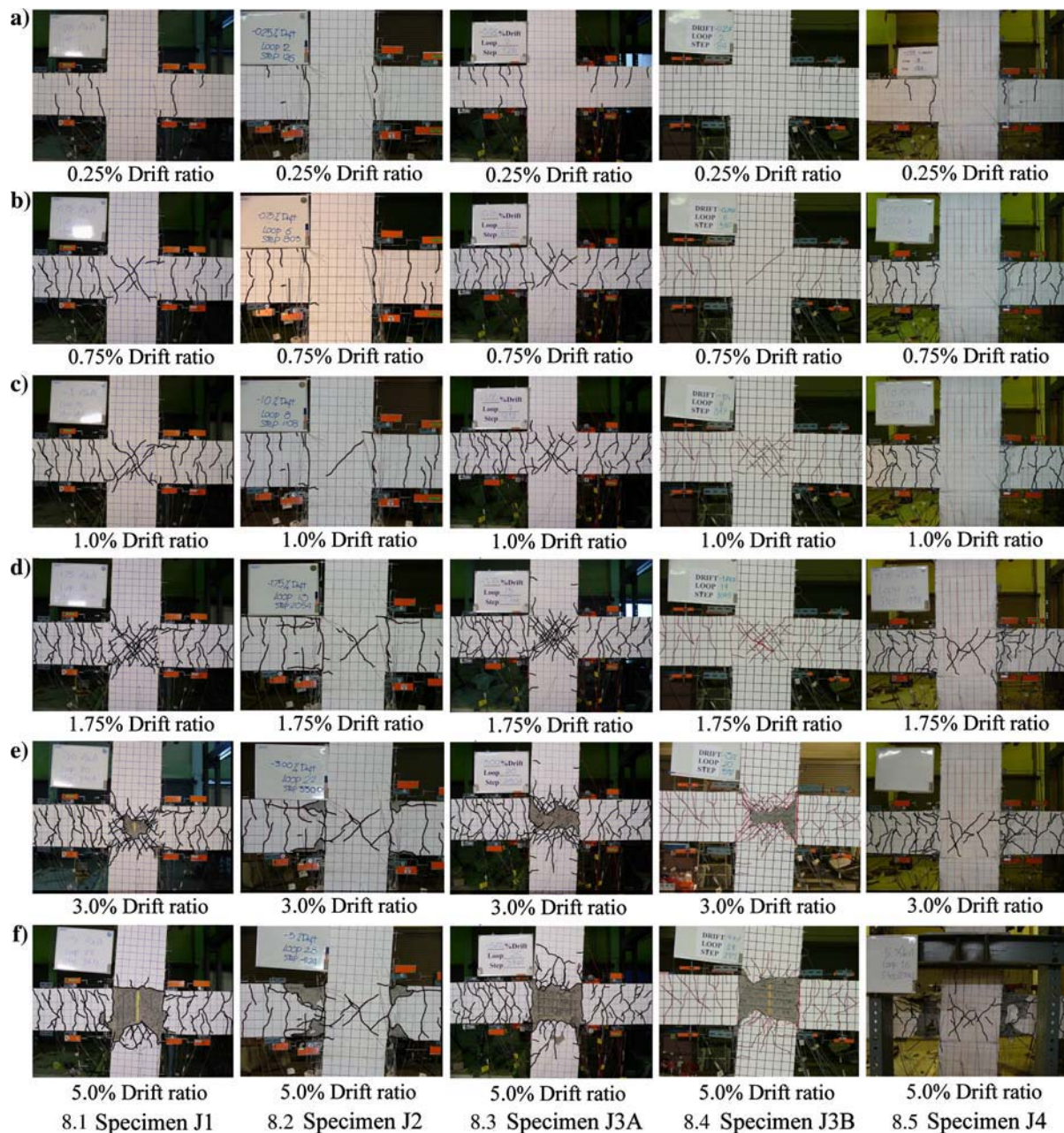
Fig. 8 Progress of cracking development of each specimen
