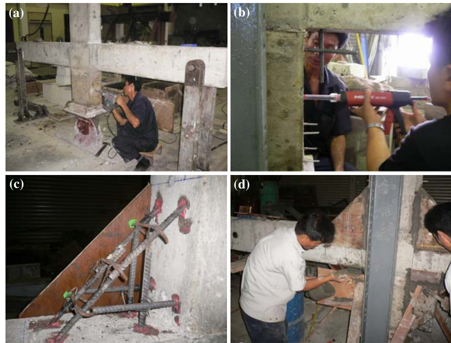
Fig. 8 Construction stages of specimen PJE2. (a) Drilling column and beam. (b) Inserting dowel bars and injecting epoxy into drilled hole. (c) Reinforcement after epoxy injection. (d) Casting concrete
