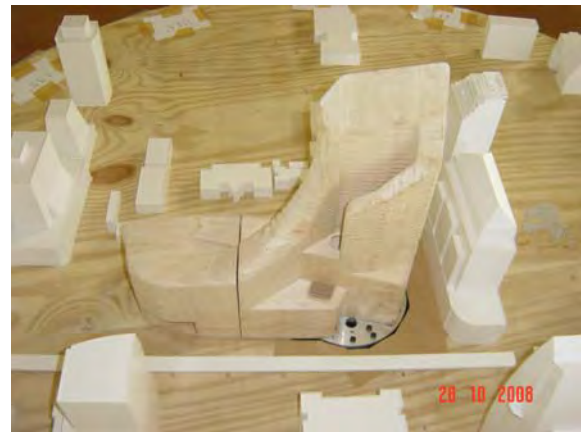
Figure 11. High-frequency force balance model of Central Man-U building in Bangkok
