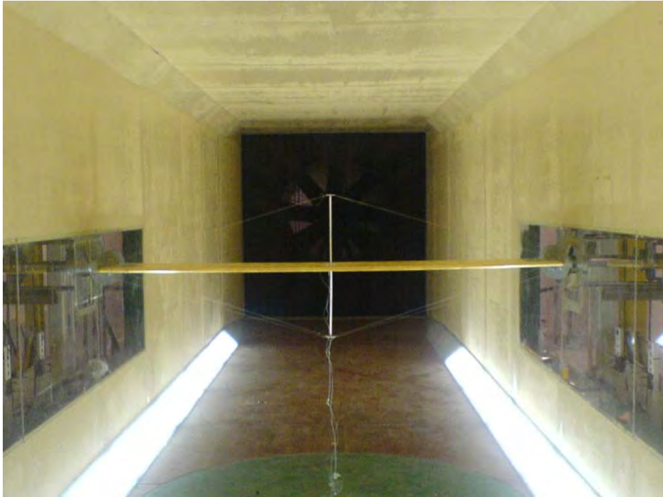
Fig. 7.15(a) Thin flat plate model with king-post in wind tunnel : static test setup
