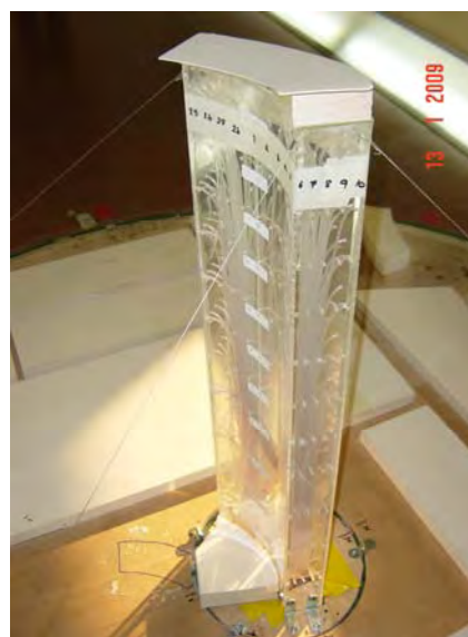
Figure 7. Rigid model of Knightbridge building in Manila
