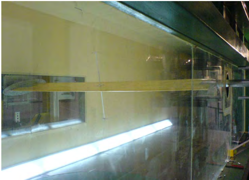
Fig. 7.15(a) Thin flat plate model with king-post in wind tunnel : static test setup
