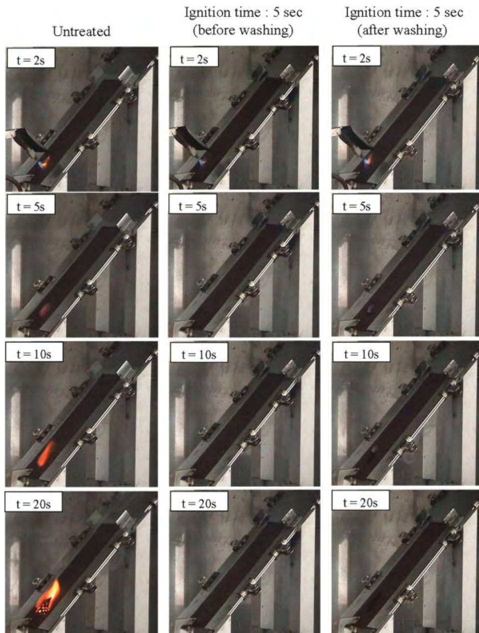
Figure 12 Flame spread test of untreated cotton fabric and treated cotton fabrics (before and after washing). [Color figure can be viewed in the online issue, which is available at www.interscience.wiley.com .]
